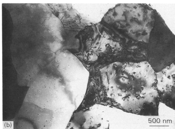
Figure 2 (a) Optical micrograph of 8090 base metal in the unetched condition and taken from a transverse plane. Intermetallic phases are seen in the aluminium matrix; (b) A transmission electron micrograph of 8090 base metal in the as-received condition showing the sub-grain structure.
